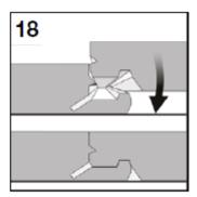
Insert a second panel lengthwise into the groove profiling of the preceding panel areas and slide it to the left at an angle of 20 ° to the already laid panel. Then bend downwards and snap in with pressure from the top to the audible click. Care must be taken to ensure that the panel to be laid is inserted and guided cleanly in the longitudinal profile.
