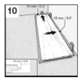
Start laying in the left corner of the room. Place the first panel with the spring side to the wall and secure the edge distance with spacer wedges. Absolutely maintain a 12-15 mm edge distance (expansion joint) to the wall, heating pipes, pillars, door stoppers etc.
