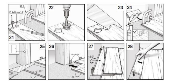
For heating pipes, holes that are 3 cm larger than the pipe diameter must be recessed. Saw out, glue, fit and fix with a wedge until the glue has hardened. Then cover recesses with radiator cuffs. Shorten the wooden door frame so that a panel with impact sound insulation incl. 2 - 3 mm distance below it fits. Remove spacer wedges after installation.
