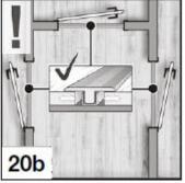
For installation surfaces with a length of more than 8 m or width and in strongly crooked rooms, expansion joints (at least 2 cm wide) are required. Only then can the soil expand or contract as the climate changes. Please note this also for a cross-room installation. Here, the areas in the door frame area must be interrupted. Expansion joints can be expertly covered with appropriate profiles.
