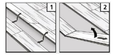
The disassemble over the floating floor follows that firstly the entire row of the panels are removed at the long sides through bending the Lock. Afterwards the planks are bent head-flat on the floor at the narrow side and the connection is released.
